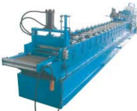
roll forming machine (350mm interlocking door panel) reference figure
