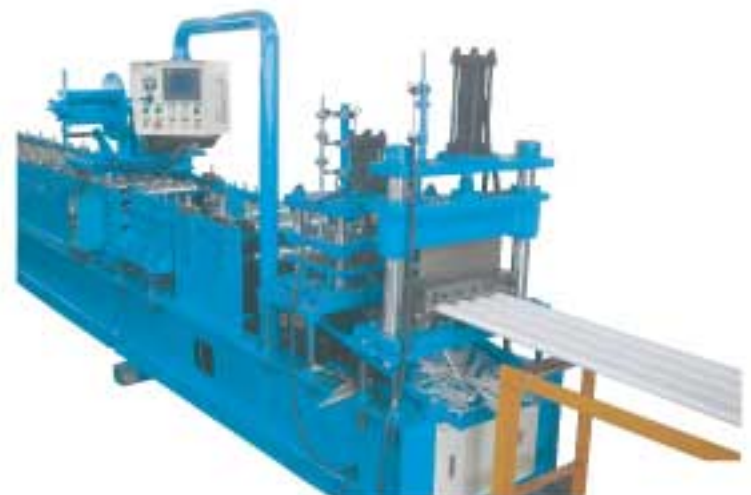
roll forming machine (350mm interlocking door panel) reference figure
